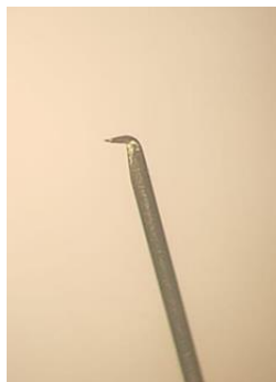
Figure (6): The modified hypodermic needle showing the sharp near 90 degree bent (right) with smooth outer surface (left)
